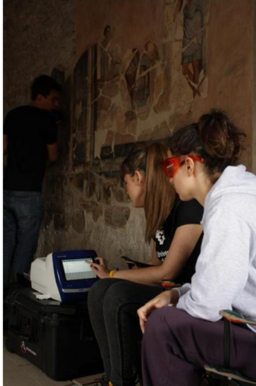
Fig. 1: A detail of the iRaman Pro spectrometer use in the House of the Gilded Cupids (Casa degli Amorini Dorati).
