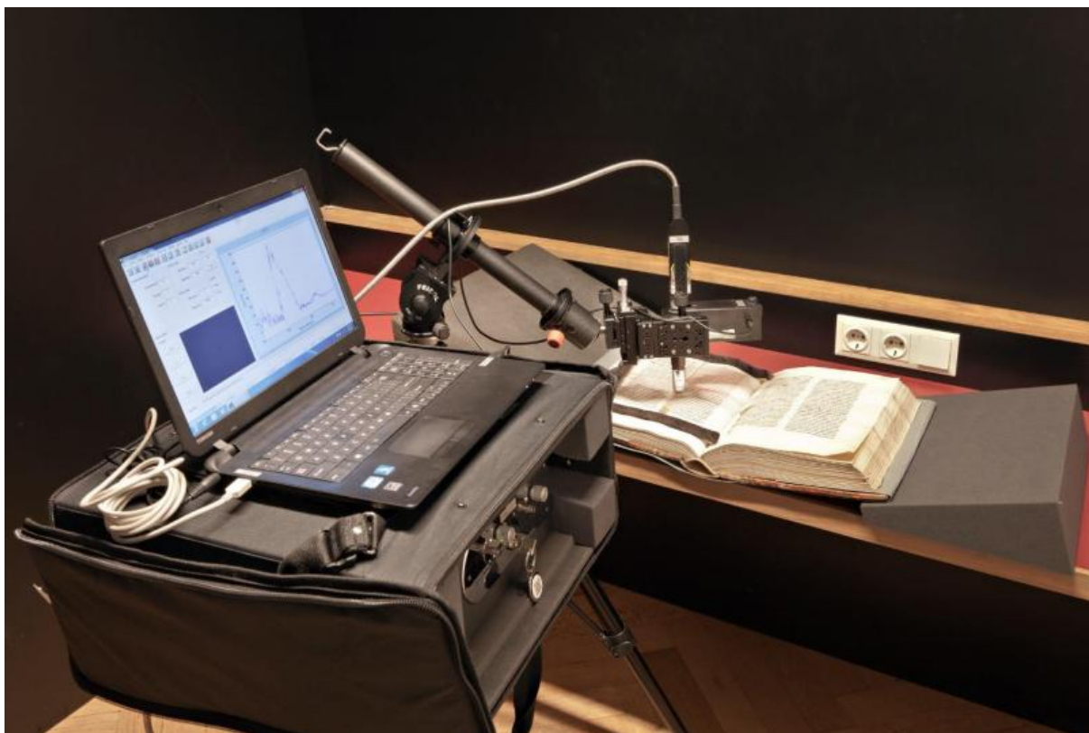
Fig. 1: Raman analysis of a Greek manuscript in the Austrian National Library in Vienna, Austria.
