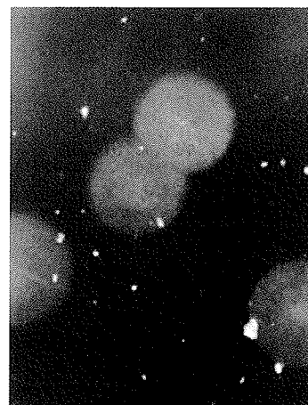
Figure 4. Phase separation and crystallisation of surfactants in an acrylic waterborne coating. Magnification x45.
