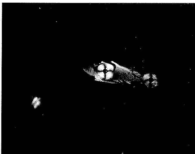
Fig. 10: Microscopic image, crossed polars, starch in red paint
