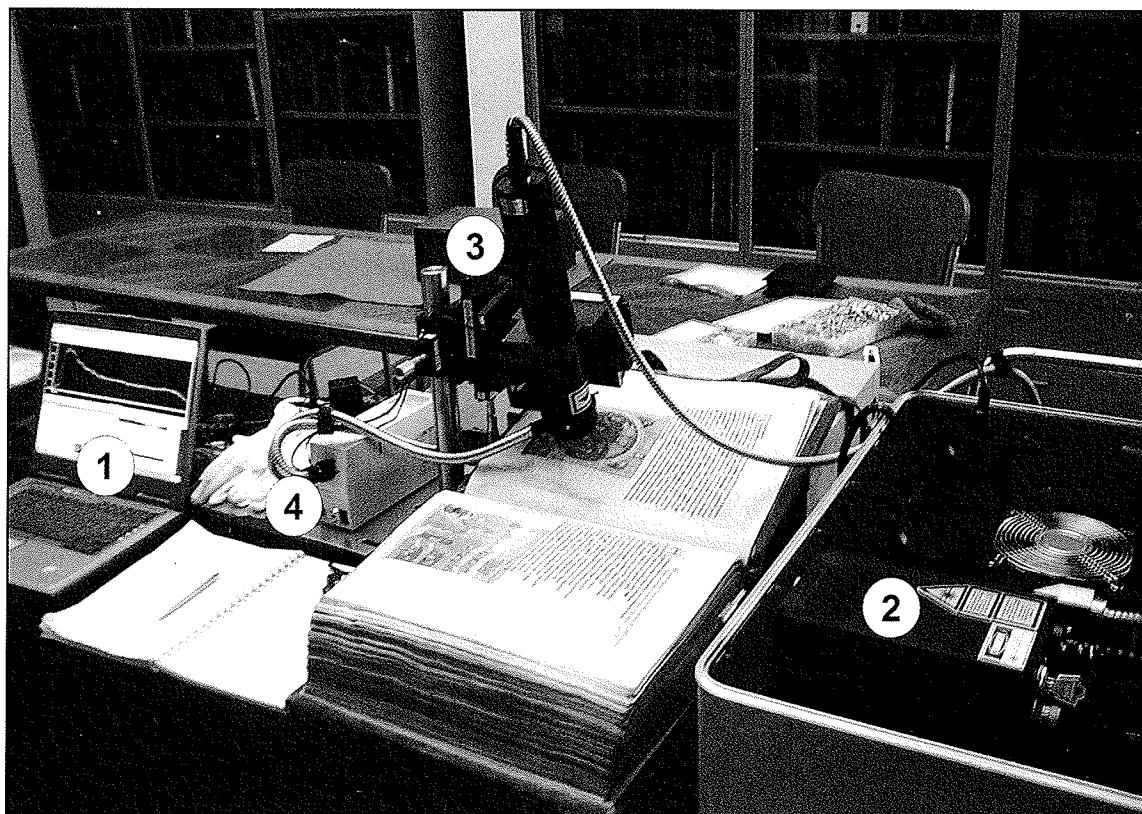
Figure 1. The Mobile Art Analyser (MArtA) set up in the library of Ghent University, during direct analysis of a mediaeval Mercatellis manuscript. 1: notebook computer that is connected to the spectrometer by USB coupling; 2: mobile spectrometer with the diode laser mounted on top; 3: probe head mounted on a vertical post and micro positioners to enable focussing on the manuscript; 4: fibre optics coupled white light source for visualisation of the area under examination.
