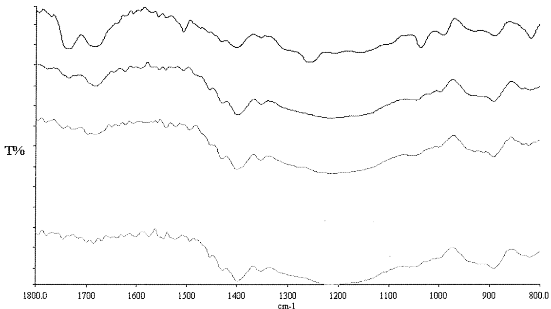
Fig.6 – sequence of spectra of Akeogard ME: after 1 day (top), 4 days, 8 days, 11 days, 58 days (bottom)
